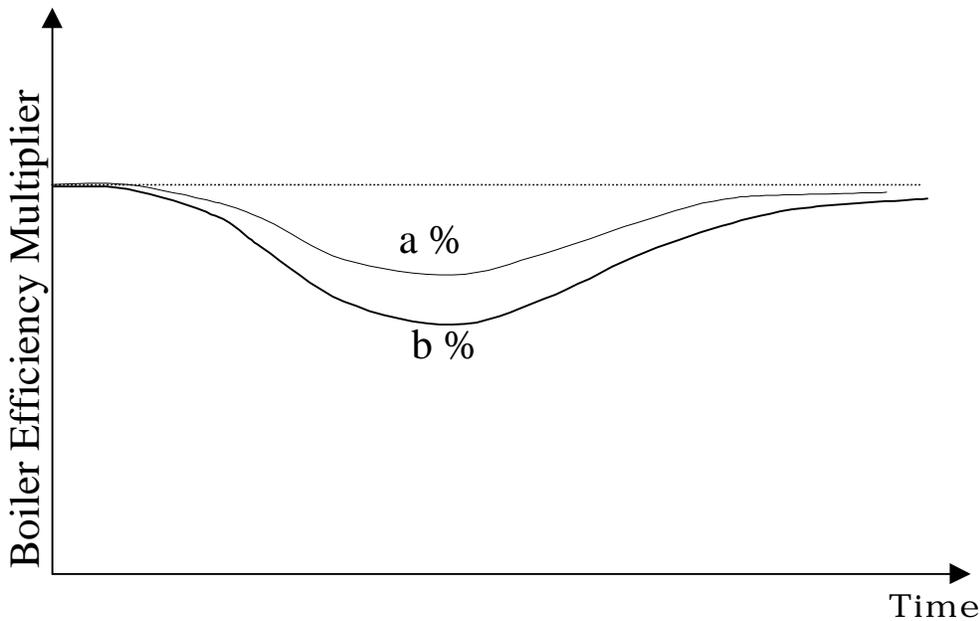
**Figure 1.** Graph of the boiler efficiency curve following a step generation change request of **a%** or **b%**, where **b > a**, applied at origin.
